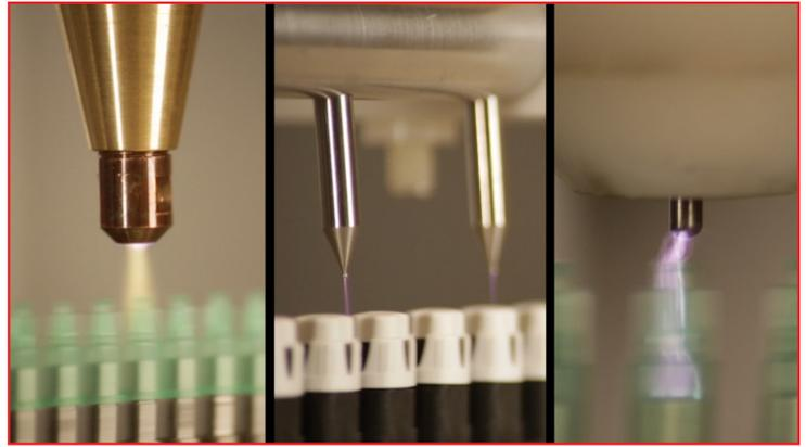
The NeedleTEC station is a compact, self-contained tabletop Corona System that includes a microprocessor-controlled generator, transformer, electrode assembly and ozone filter. The NeedleTEC station is installed in front of the adhesive applicator station on assembly lines, and treats all standard needle hubs as well as customized hubs.
