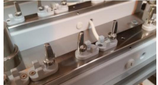
32 injection molded parts needed to be systematically and simultaneously checked across a single plate. The cycle times and quantity of components undergoing simultaneous testing ruled out the use of conventional flow and pressure decay tests.
